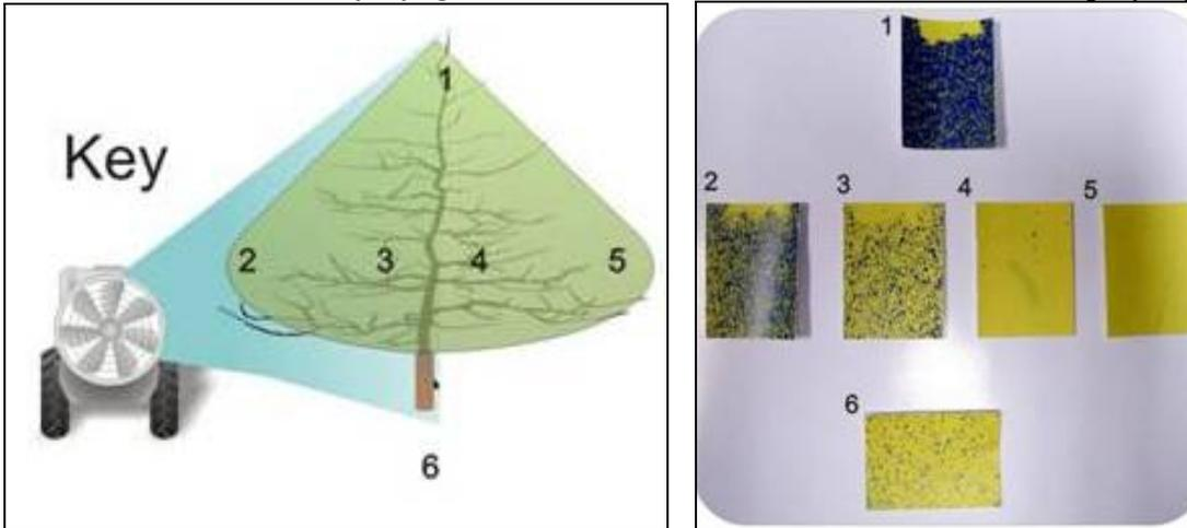
Left: Place at various locations on the tree, including on the ground (drawing from Jason Deveau). Right: The card is wet closest to the sprayer, adequate in the middle of the tree and dry on the opposite side of the tree. The card on the ground shows some blue colour from dripping, but not excessive. In this example, it will be necessary to spray from both sides of the tree to ensure adequate coverage.
