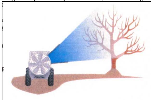
Pictures above: Adjusting nozzles to match the target (drawings from J. Deveau).
