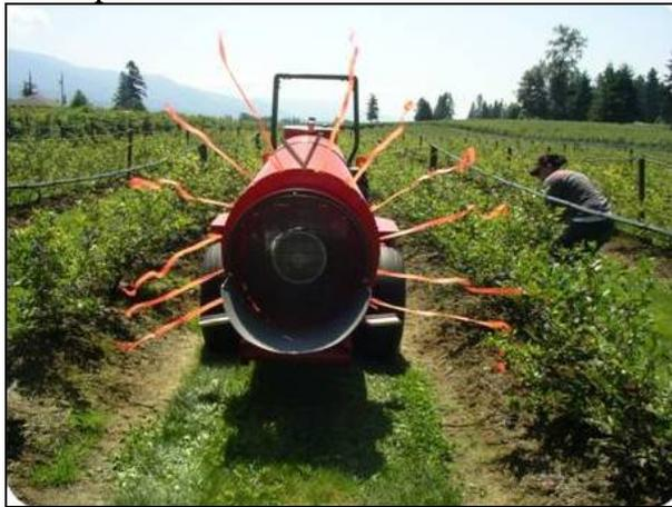
Left: In spring, if too much wind is produced, the spray will blow through the plant instead of settling. Right: Short ribbons (25-cm length) are attached at each nozzle position to show air direction. Nozzles that are not required should be turned off or oriented to match the target shape.
