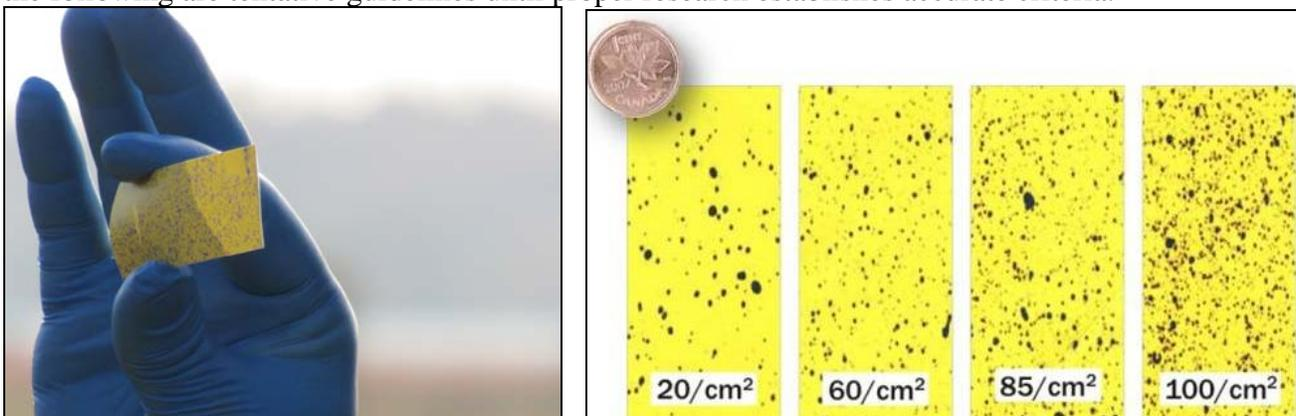
Above left: The cards can be cut into strips. Wear gloves to prevent contact with skin oil or sweat. Right: 85 droplets per cm<sup>2</sup> with total coverage of 10 to 15% should be sufficient for most foliar sprays. Below 85 droplets/cm<sup>2</sup> is likely not sufficient coverage, over 85 droplets is likely more than necessary.
