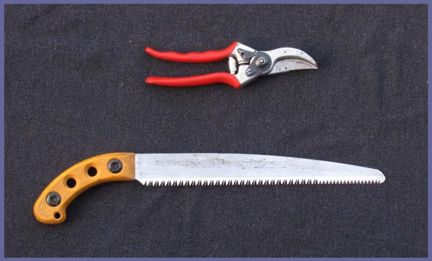
Top: Pruning shears (secateurs) are preferred for small diameter branches. Bottom: A pruning saw is a better tool when working on larger branches. Not shown: Loppers are used to prune shrubs and remove fruit tree suckers.
