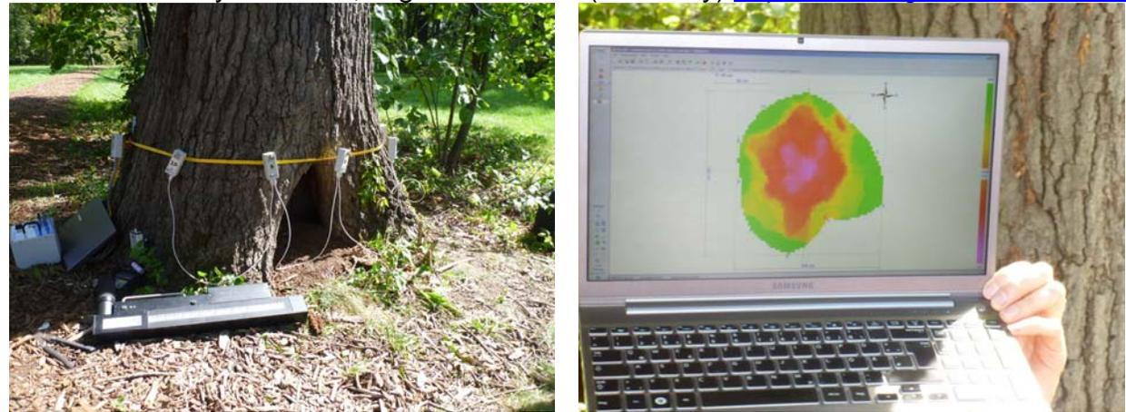
Left: Sensors are attached around the trunk and send signals to each other.
