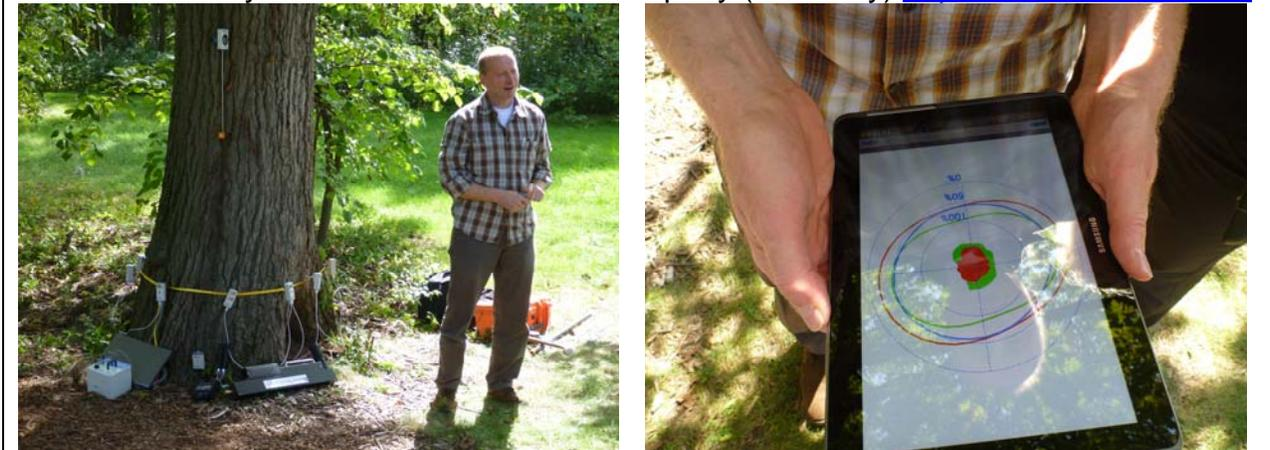
Left: Sensors attached around the trunk send signals to each other.
